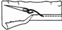
Figure 3. Turn Edge Under and Sew.
